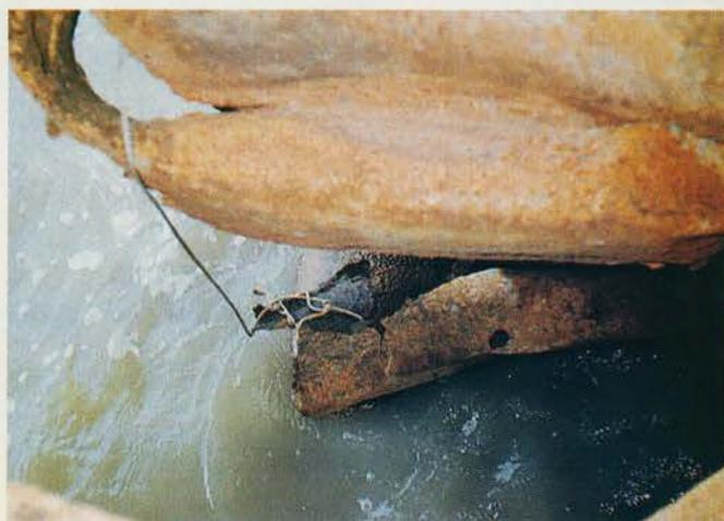
**FIGURA 4. PARTE DA ESTRUTURA DE NAVIO, QUEBRADA POR CAUSA DA CORROSÃO.**
